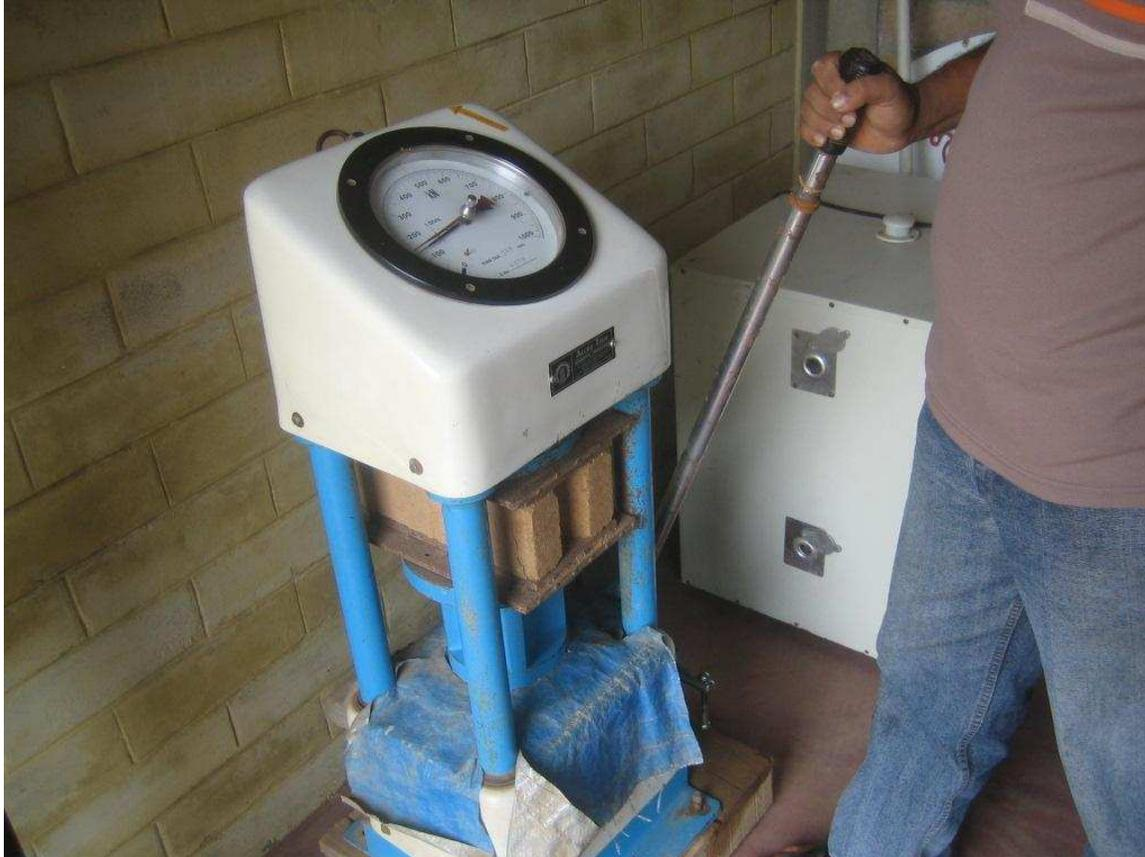
**Compressive Strength Testing Machine**
